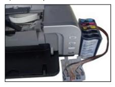
Put the CIS at the right side of printer And make sure the tube line does not twist.
